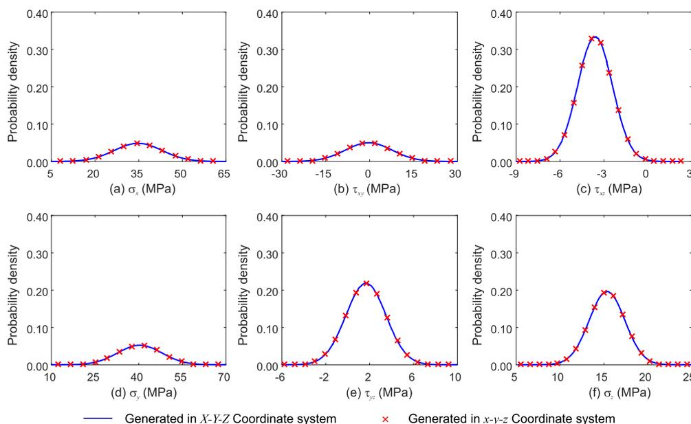
**Fig. 6.** Probability density distributions of tensor components generated by the proposed fully tensorial approach in both  $X$ - $Y$ - $Z$  and  $x$ - $y$ - $z$  coordinate systems, and transformed into a common  $x$ - $y$ - $z$  coordinate system.
