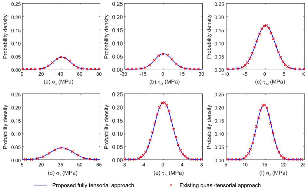
Fig. 3. Probability density distributions of tensor components generated in the  $X$ - $Y$ - $Z$  coordinate system by both the proposed fully tensorial and existing quasi-tensorial approaches.
