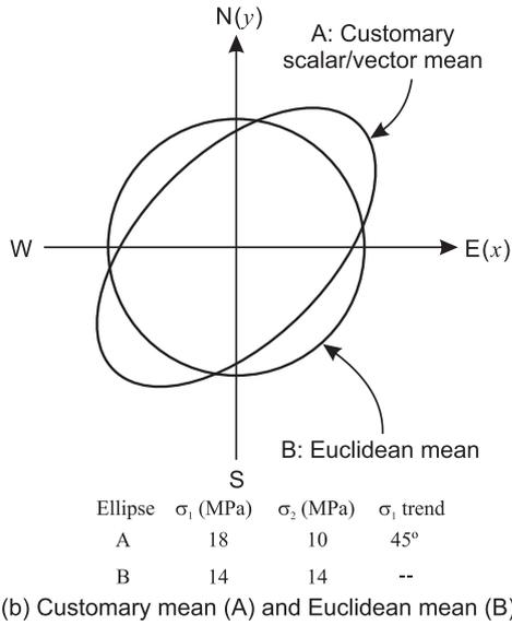
Fig. 2. Demonstration of stress tensor averaging using customary scalar/vector and tensorial approaches (after Dyke et al.<sup>29</sup>).
