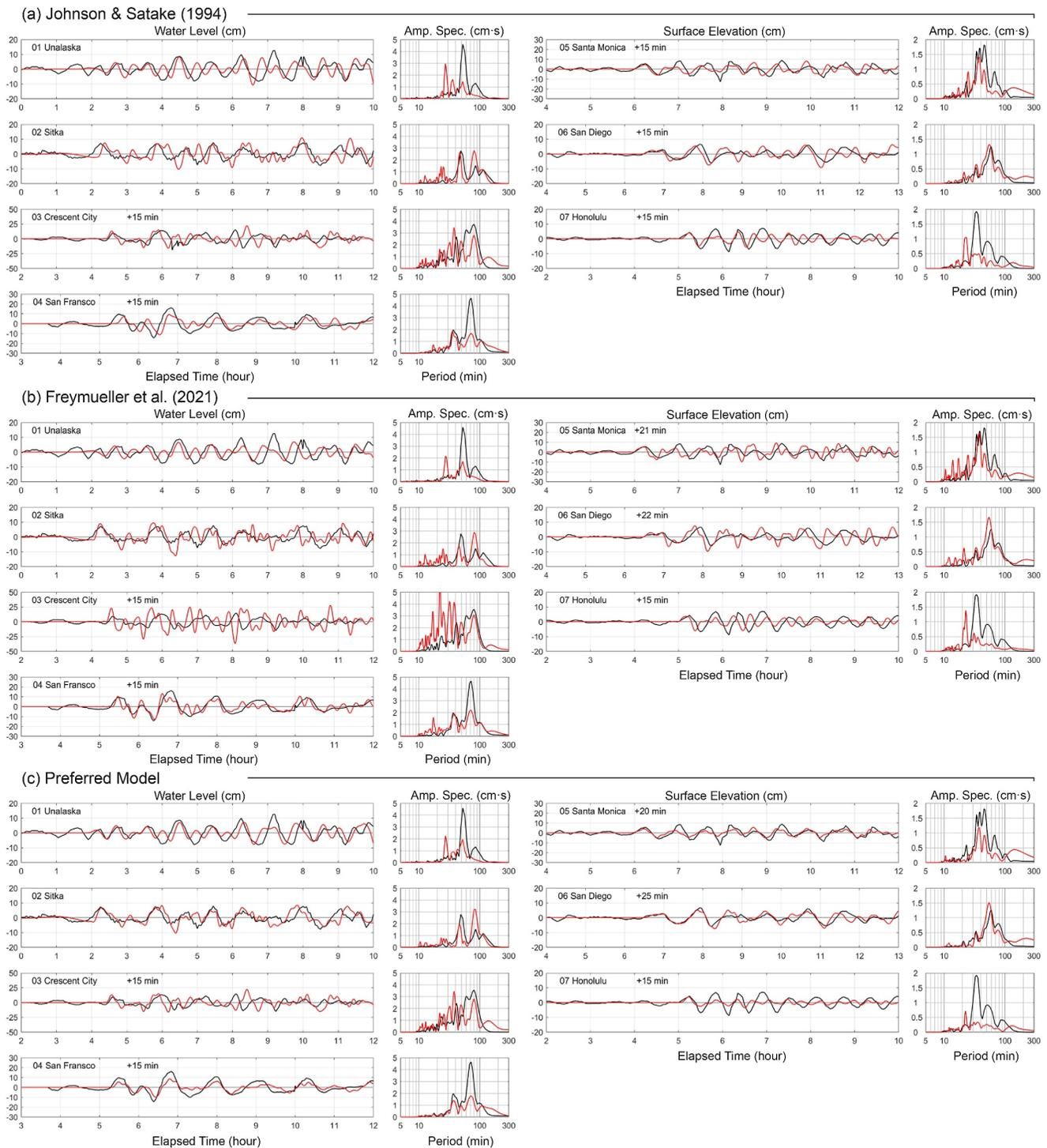
**Figure 4.** Comparison of observed tsunami waveforms and spectra (black lines) from the seven tide gauge stations in Figure 2 with corresponding calculations for the three slip models for the 1938 event in Figure 3 (red lines). Time shifts of the indicated amount have been applied to the computed tsunami signals at large distances.
