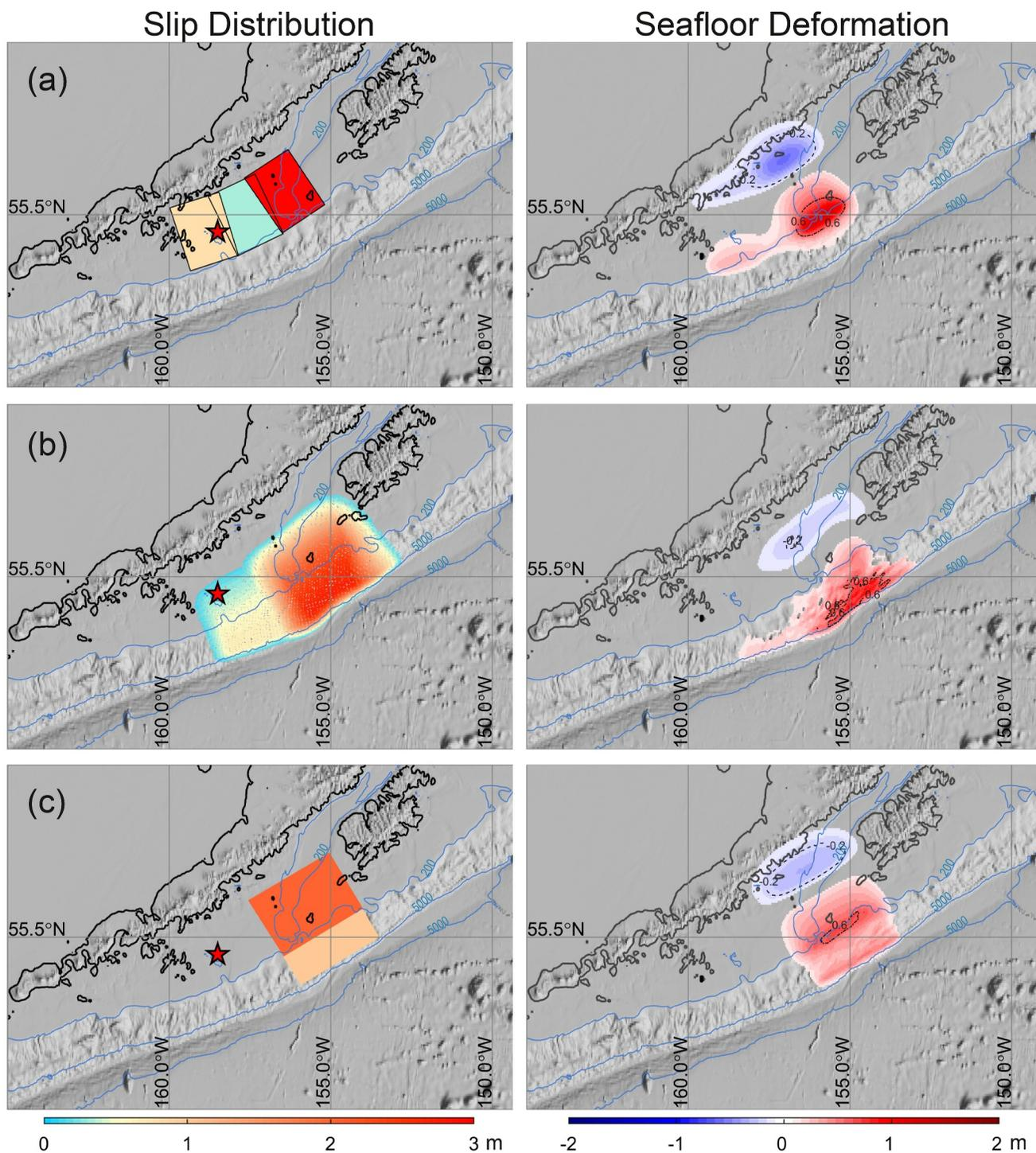
**Figure 3.** 1938 earthquake slip distributions (left column) and computed seafloor deformation (right column) for the models of (a) Johnson and Satake (1994), (b) Freymueller et al. (2021) far-east, and (c) the updated preferred 1938 model in this study, which has only 1 m of slip beyond the shelf break and less uplift of the continental slope in contrast to 3 m of shallow slip in the Freymueller et al. (2021) model.
